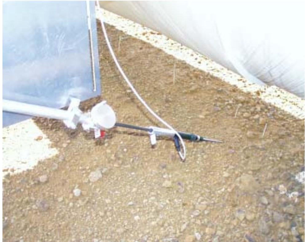
Figure 4: Instrumented Prodder under test with the manually operated spindle
