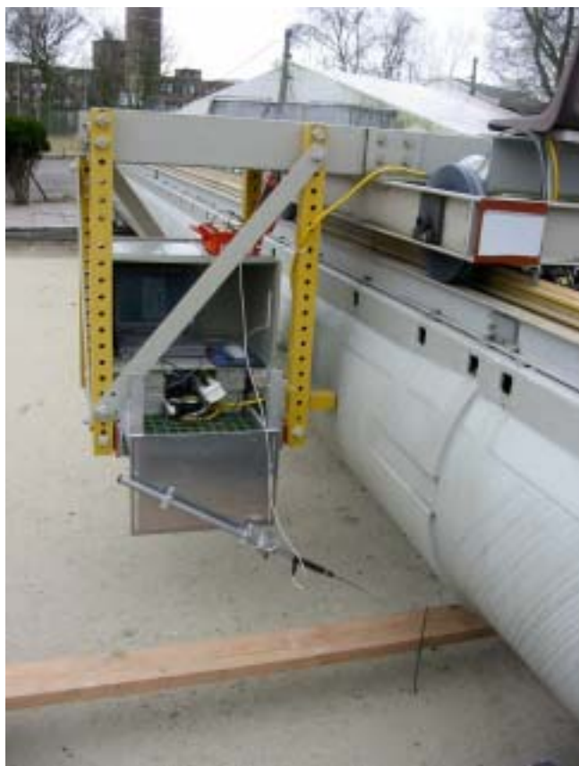
Figure 3: Instrumented Prodder mounted on the measurement platform
