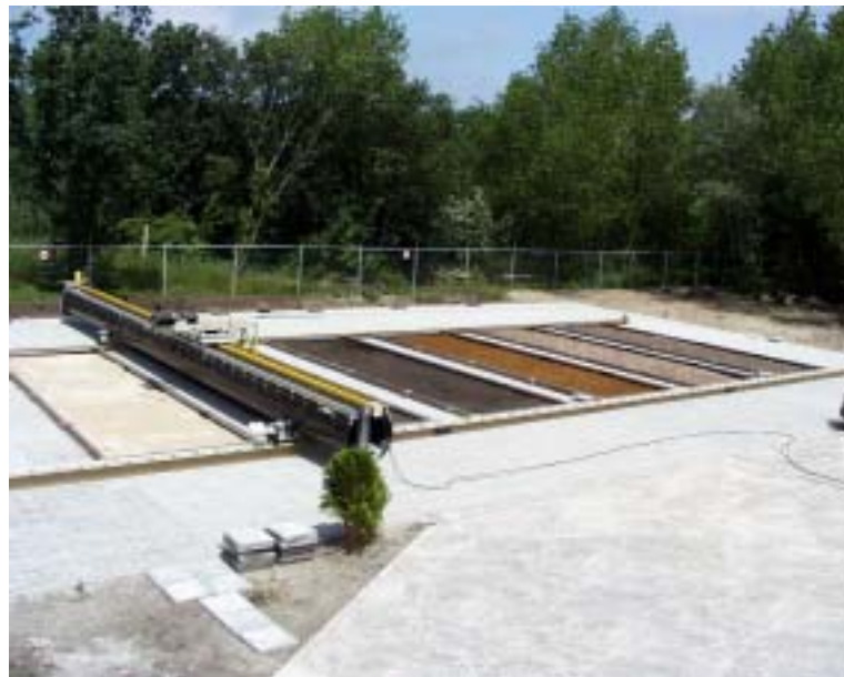
Figure 2: TNO-FEL outdoor test facility consisting of 6 test lanes and an XY-positioning frame
