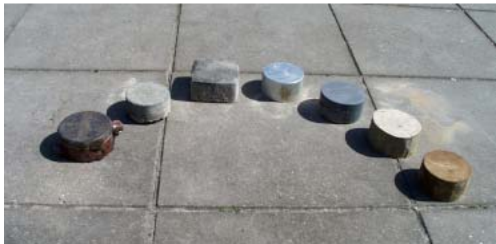
Figure 8: Seven different target types. From left to right: inert PMN, concrete, brick, aluminium, PVC, wood, steel.
