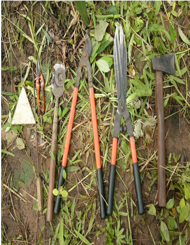
Figure 2 The CMAC manual demining toolkit. The ring-magnet in use by CMAC is attached on the excavation tool on the left. The Minelab F1A4 metal detector is not shown.
