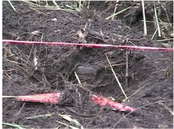
Figure 2: PMN6 AP mine in Kamrieng minefield shown uncovered prior to detonation
