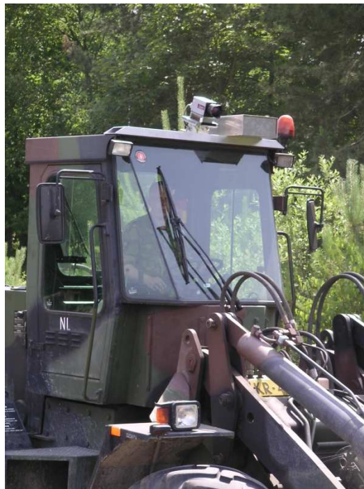
Figure 3.1 Polarisation camera mounted on the wheel loader. The metal box right of the camera contains the computer.
