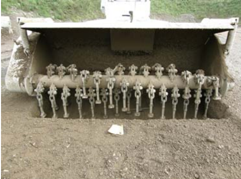
Figure 39: Placed AT mine m/41-47 in front of flail.
