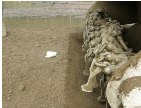
Figure 40, Placed AT mine m/41-47 in front of flail
