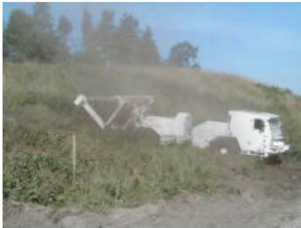
The pictures show clearing in 20% upward slope
