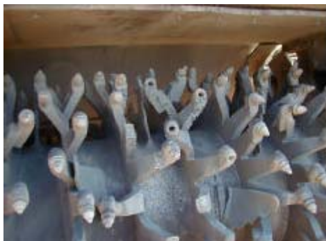
The picture shows the clearing roller where the mine was detonated
