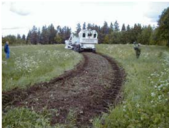
The picture shows minimum turning radius test
