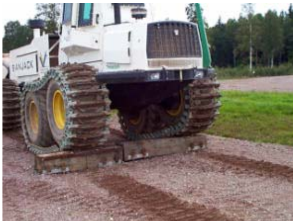
The picture shows backwards obstacle test
