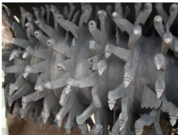
The picture shows damages caused by strv 5 on the clearing roller
