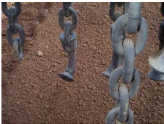
The pictures show damages to the clearing tool after carrying out the test
