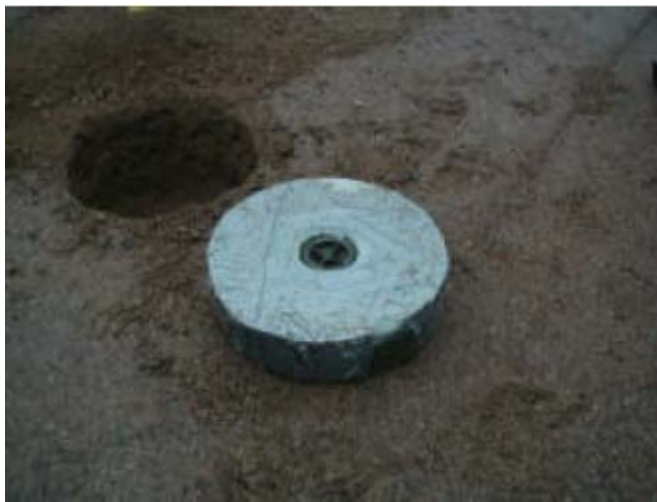
The picture shows strvmina 5 reinforced with nylon sheet compacted with fabric tape
