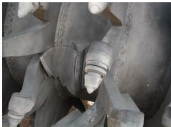
The picture shows damaged shark fin
