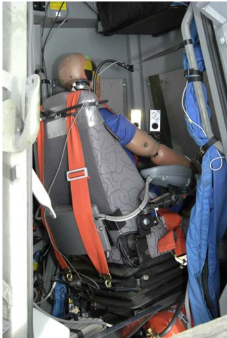
Figure 2: Crash dummy Hybrid III in driver's seat.
