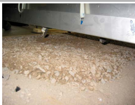
Figure 16: Targets Covered with 2 cm of Gravel
