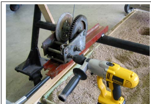
Figure 2: Winch Mechanism to maintain 180 m/h
