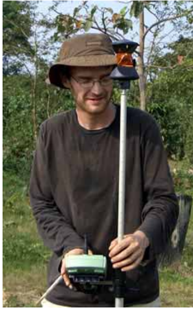
Plate 5-1 Operating the Station remotely
