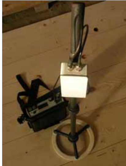
Plate 12-2 Bartington MS2D configuration
