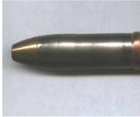
Plate 3-2 Projectile of 20mm cannon shell (from website of Colin Stevens, Burnaby Village Museum, Canada )
