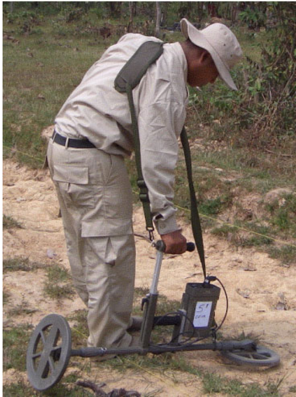
Fig.: 8 CEIA Mil D1/DS double-head UXO detector under test in the STEMMD Laos trial
