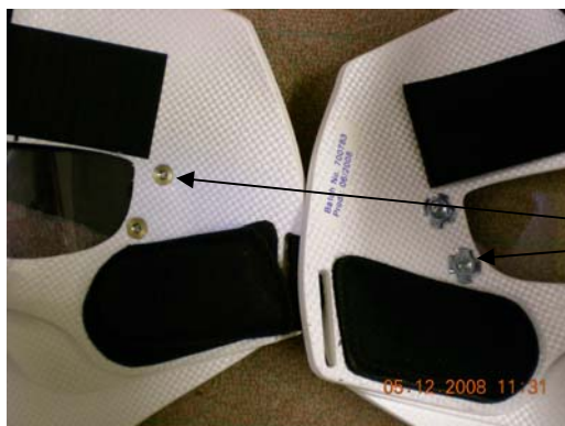
Inside view: Threaded rivets imbedded in the composite (new mask on the right hand side)
