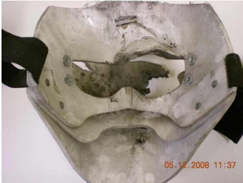
Mask seen from the inside with severe damages.
