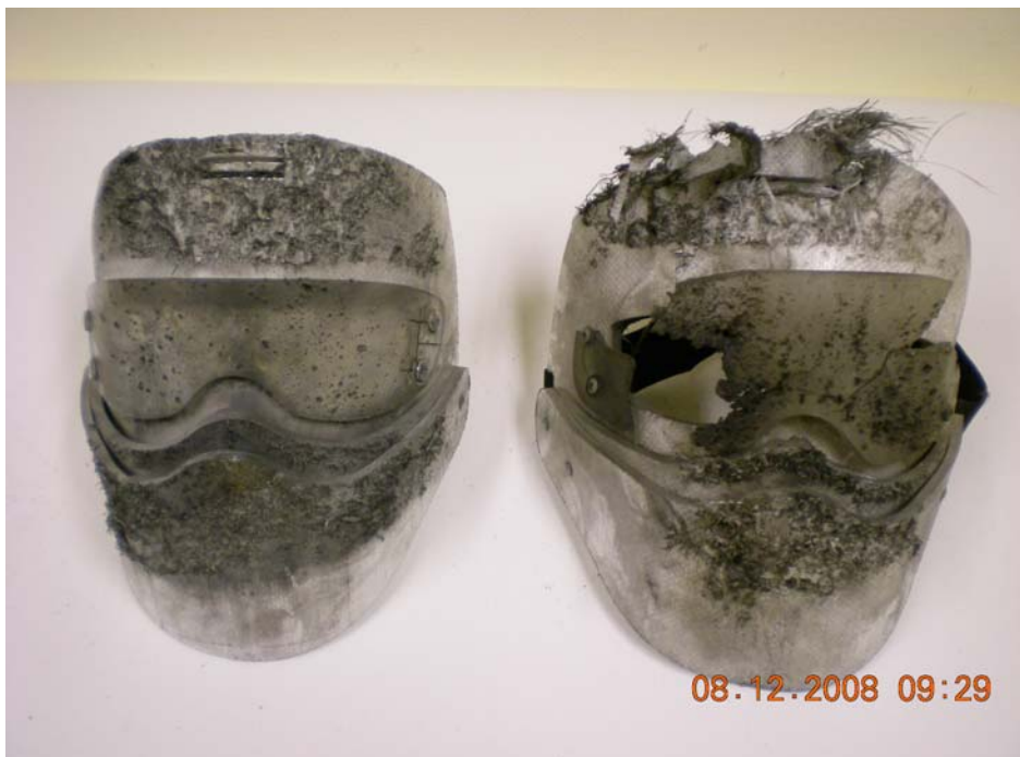
Left: Face mask from first blast test using 140 g TNT equivalent (m/46)
