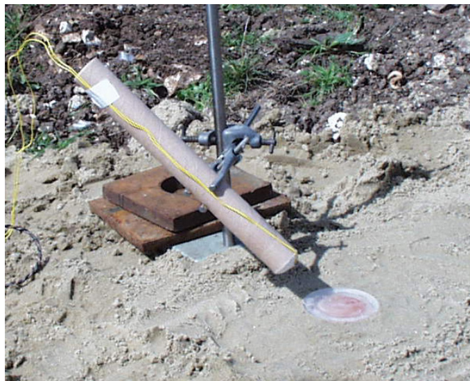
Figure 3. Photograph of a Buried Simulated Mine with Torch Positioned for Firing.
