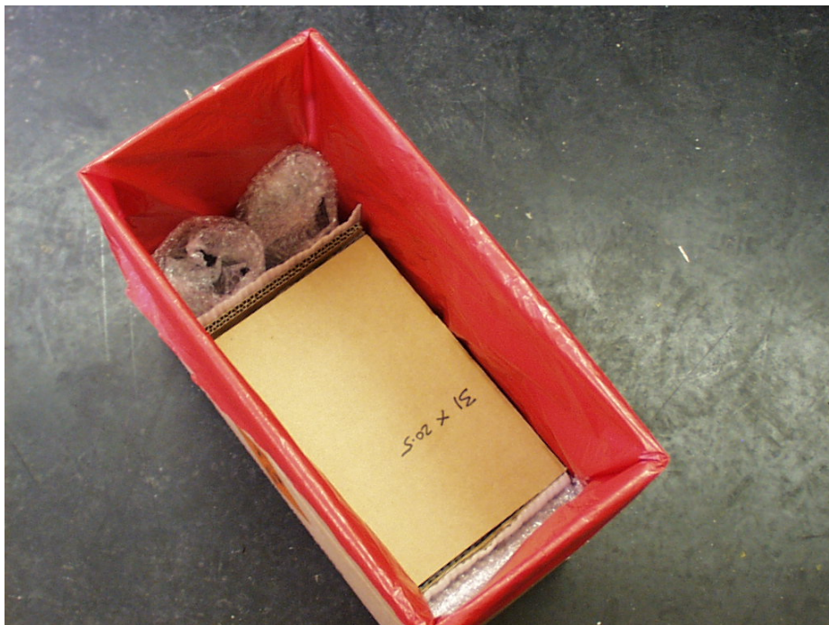
Figure 7. Plastic Containers of First-fire and Fuzeheads at One End of the Package.
