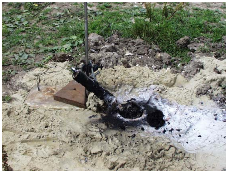
Figure 4. Example of a Burned Out Mine (No Detonator Present).
