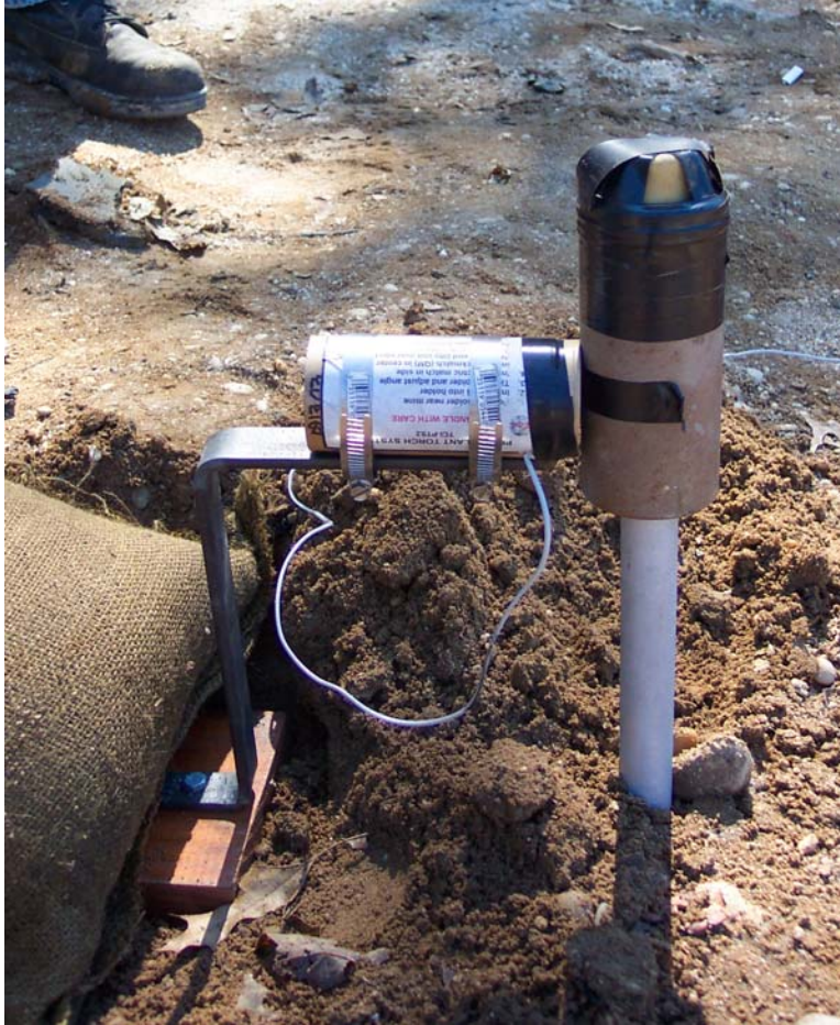
Figure 4. Placement of Torch for Stake Mine Neutralization.
