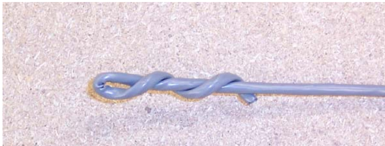
Figure 2. Picture of Twisted Wire Illustrating the Igniting Cord Configuration for Torch Initiation.
