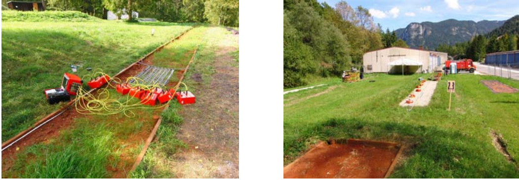
Fig. 2: Test lane 1.1 “Laterite“ with geoelectrical measuring array, viewing direction North (left hand). Training lane 1.3 “Laterite” in the front and lane 2.3 “Magnetite/Sand” in the picture center, viewing direction East (right hand).
