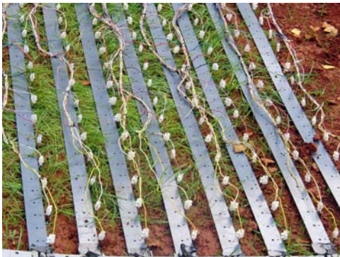
Fig. 17: Geoelectrical measuring array in test lane 1.1 “Laterite”.
