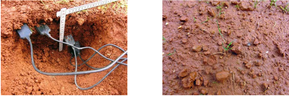
Fig. 6: TDR probes in test lane 1.1 “Laterite” before being buried and view of the soil surface.
