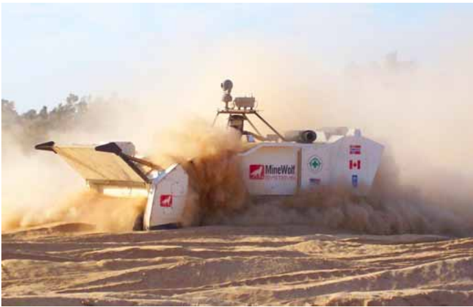
Mini MineWolf with remote camera during demining operations in Jordan
