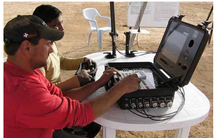
Remote operation of the Mini MineWolf using Remote Video Guidance System
