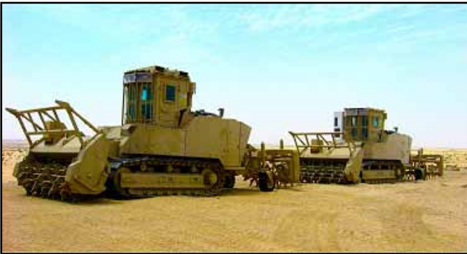
MineWolfs with Lifter attachment for bringing mine fragments to the surface for visual inspection and removal
