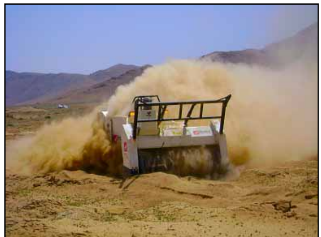
DDG Mini MineWolf during demining operations in Afghanistan
