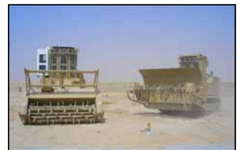
MineWolfs with both tiller and flail attachments. The white cabin attachment (left) allows a trainer to accompany the operator during training
