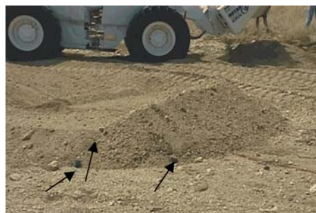
The ROTAR has backed out of the field and is ready to sift the content inside the bucket. Sand is constantly falling out of the bucket. Much of it back into the test line
