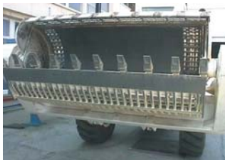
The 45 x 45 mm sifting grids clearly visible. The inner sheet steel plate is also seen on the picture
