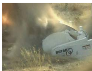
The J69 mine detonating inside the closed bucket Flames can be seen meters to front of the bucket
