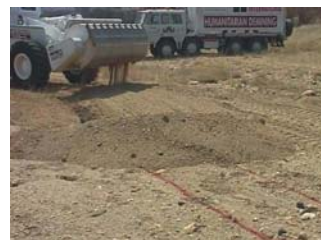
The ROTAR has backed out of the field and is ready to sift the content inside the bucket. Sand is constantly falling out of the bucket. Much of it back into the test line
