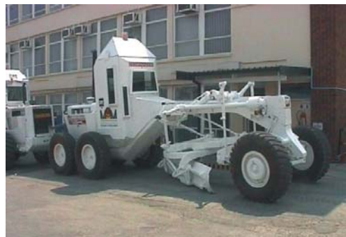
The new MgM grader. The mine protected cabin is similar to the cabin on the MgM ROTAR
