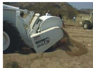
The rotor is lifted and closed. More sand escapes from the rotor
