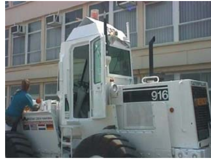
Armoured plates can be seen on the sides of the machine. The black antenna socket is for HF communication
