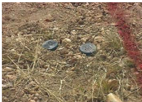
Two dummy mines placed in the test line during the first clearance test
