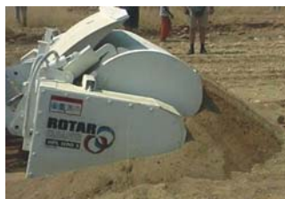
The rotor bucket being pushed into the soil thereby moving soil further to the front and to the sides
