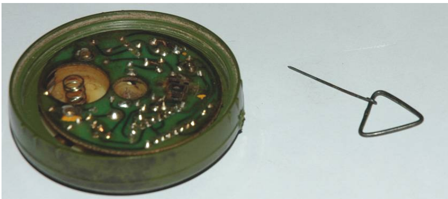
Figure 4 Type72b top casing with safety pin pulled
