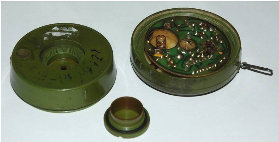
Figure 3 Type72b opened, bottom casing exterior
