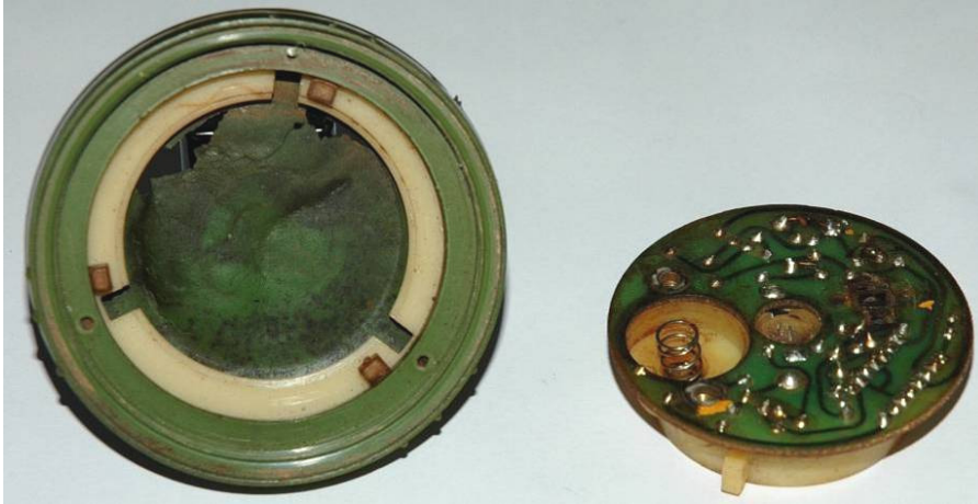
Figure 5 Type72b top casing, PCB (trace side shown) removed
