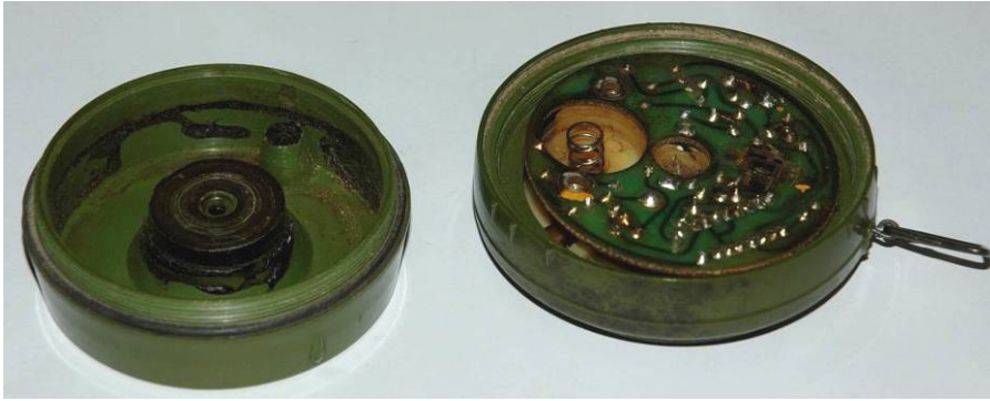
Figure 2 Type72b opened, bottom casing interior
