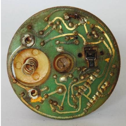
Figure 7 Type72b printed circuit board trace side
