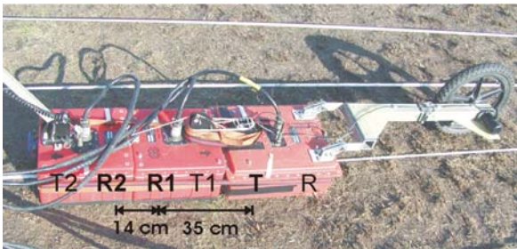
Figure 3. Setup used for the groundwave measurements. A shielded bistatic 500 MHz GSSI antenna is used as transmitter and two bistatic 400 MHz GSSI antennas are the receivers. The position of the antennas in the housings are indicated whereas the active elements are in boldface (T = transmitter, R1 and R2 = receivers).
