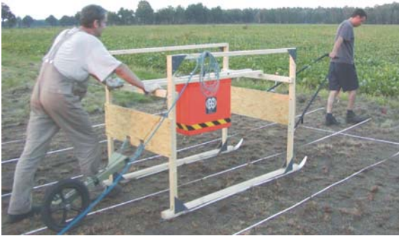
Figure 6. Measuring setup to determine the coefficient of reflection: A 1 GHz GSSI horn antenna is mounted on a sledge 0.5 m above the ground.
