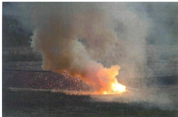
Figure 6: Typical Burning Behavior of a Thermite Hyper Heat Mine Flare
