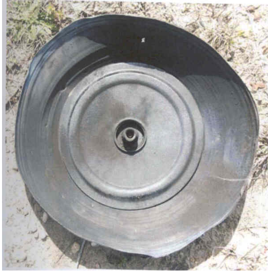
Figure 18: Interior view of the pressure plate of the deflagrated TM-46 AT mine shown above. The detonator's detonative reaction is clearly indicated by the fragment penetrations and impacts.
