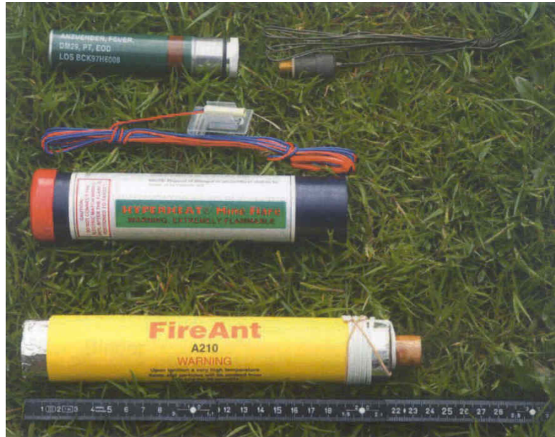
Figure 3: Comparison of the sizes of the ignition charge and (thermite) flares used
