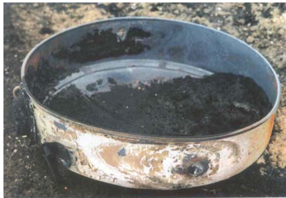
Figure 19: Lower part of the casing of a burnt out and deflagrated TM-46 AT mine (test 34), ignited by 2 FireAnt A210 placed opposite to each other
