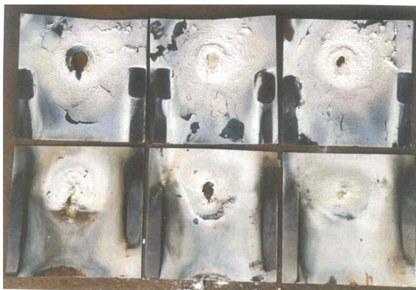
Figure 15: Penetration performance of the HMF against three laminar targets. The very thick white coating consists of aluminum oxide. The second sheet (lower row) has not been penetrated (tests 20 – 22).
