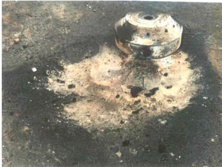
Figure 16: Burnt out TM-46 mine ignited by 1 HMF (test 43)
