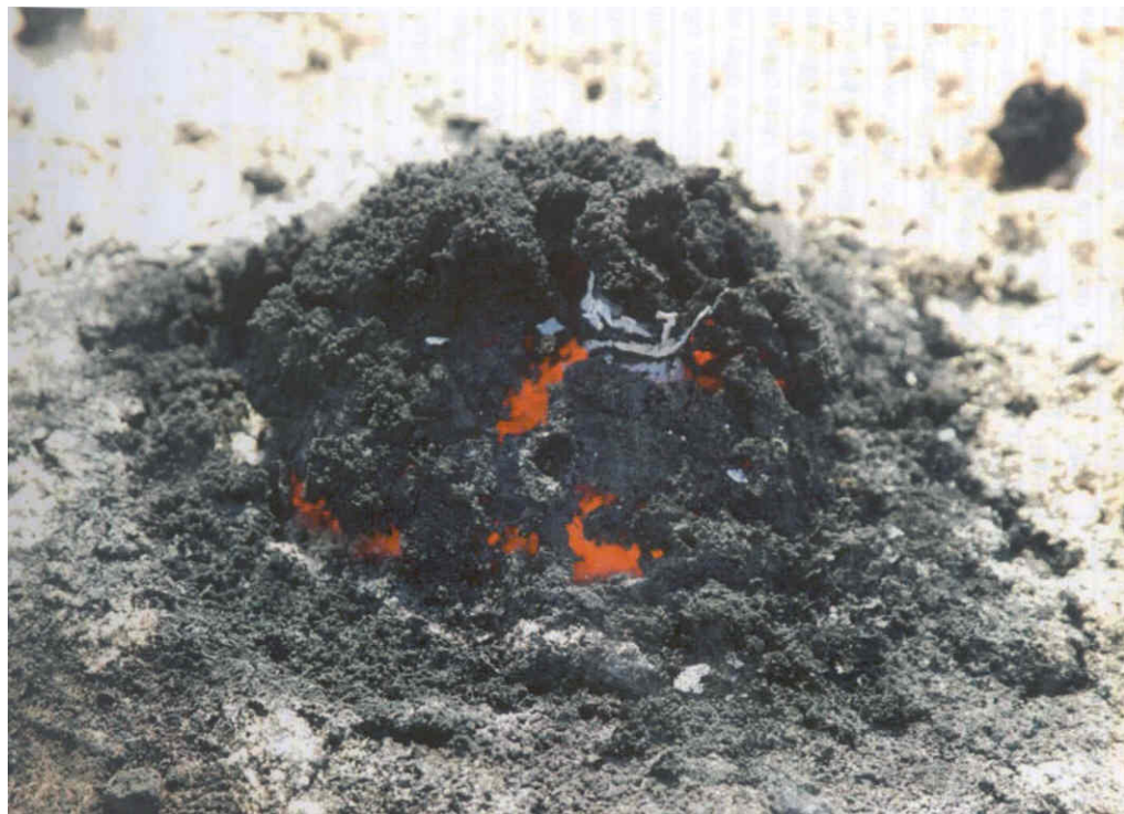
Figure 27: Combustion residues of an 8 kg TNT demolition charge (test 52), see Figure 12
