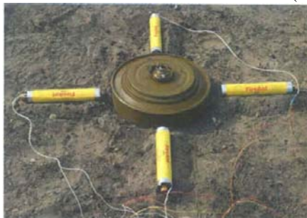
Figure 9: Surface-laid TM-46 with 4 FireAnt A210 flares (tests 38 - 42)
