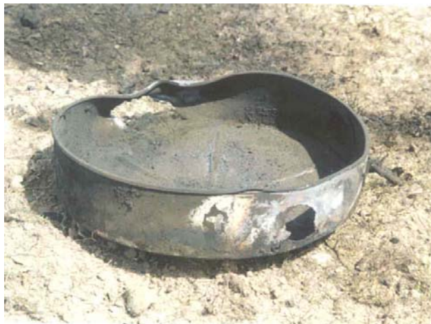
Figure 17: Lower part of the casing of a deflagrated TM-46 AT mine (test 28), ignited by 2 HMF placed opposite to each other (see Figure 10 )
