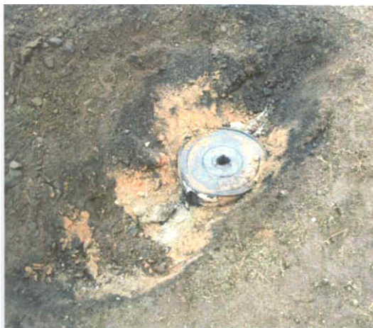
Figure 24: Remains of a deflagrated mine ignited by 2 HMF. The pressure plate was propelled away taking with it the soil covering the plate (test 54).
