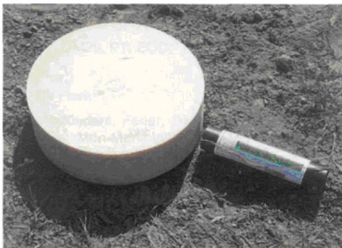
Figure 12: TNT demolition charge with one laterally positioned HMF flare (tests 51 - 53 and 55)
