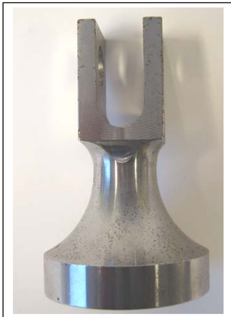
Figure 12: Short Tool Wear plate Ø 65 mm, thickness 15 mm Weight: 890 grams Material: Steel, machined, not heat treated
