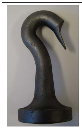
Figure 6: Mark II of Sprain Tool Wear plate Ø 65 mm, thickness 15 mm Weight: 935 grams Material: Cast Iron
