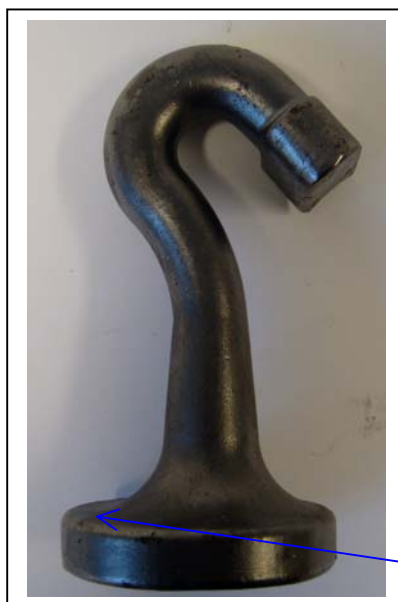
Figure 10: Mark II of Super Tool Wear plate \varnothing : Asymmetric thickness 15 mm Weight: 1000 grams Material: Cast Iron
