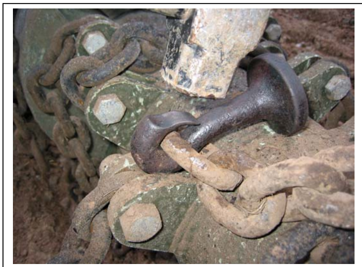
Figure 8: A sledge hammer is used in order to deform the lip
