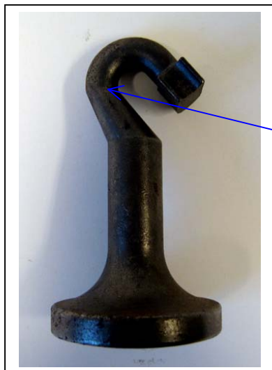
Figure 3: Mark I of MV-4 Super Tool Wear plate Ø 60 mm, thickness 10 mm Weight: 496 grams Material: Cast Iron
