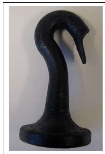
Figure 7: Mark III of Sprain Tool Wear plate Ø 73 mm, thickness 15 mm Weight: 1040 grams Material: Wrought Iron
