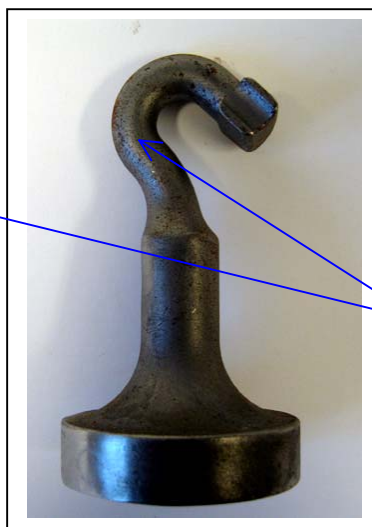
Figure 4: Mark II of MV-4 Super Tool Wear plate Ø 60 mm, thickness 15 mm Weight: 577 grams Material: Cast Iron
