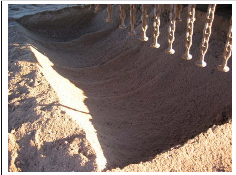
Figure 16: Evidence of ridges at the rear flail after a test in the sand lane
