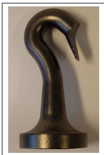
Figure 5: Mark I of Sprain Tool Wear plate Ø 65 mm, thickness 15 mm Weight: 884 grams Material: Cast Iron
