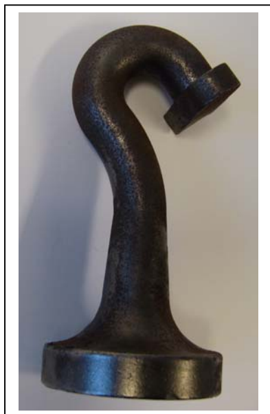
Figure 9: Mark I of Super Tool Wear plate \varnothing 65 mm, thickness 15 mm Weight: 910 grams Material: Cast Iron
