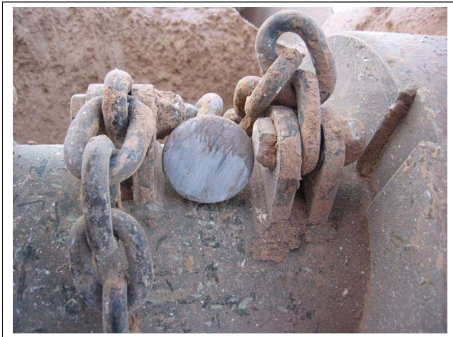
Figure 13: Wrought iron Sprain Tool Ø73 mm stuck in the attachment to the flail axle
