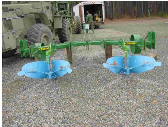
Figure 28: Bed Formers Installed on the Soil Loosener Frame
