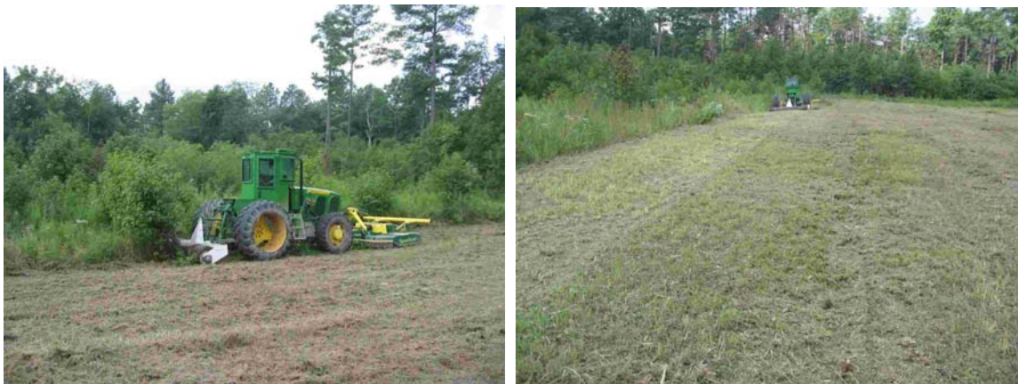
Figure 20: Area Reduction Roller and Mower Results
