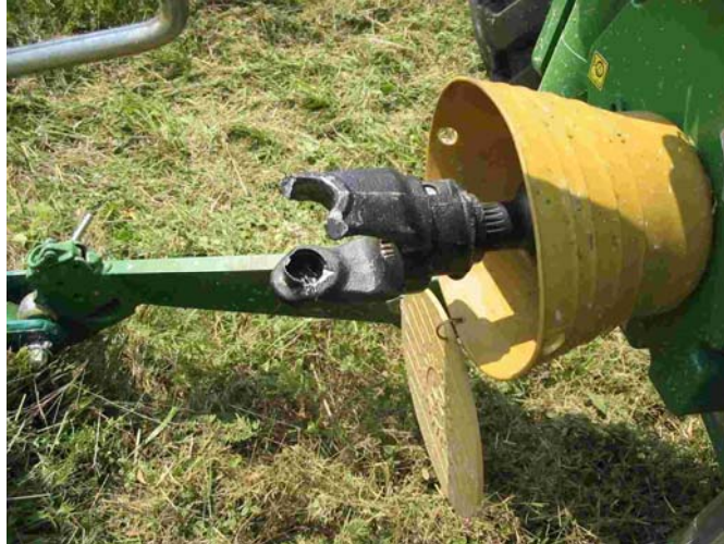
Figure 21: Sheared Universal Joint
