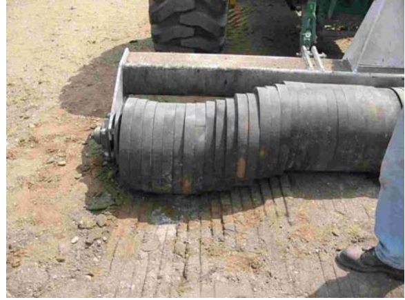
Figure 23: Results of Blast Test Against Roller
