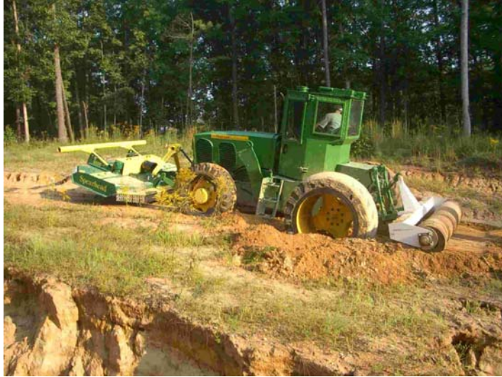
Figure 19: MCSV Stuck in Damp Sand Hill
