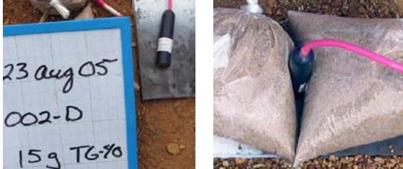
EHP Test charge # 002-D: 15 grams of TG-40 explosives (TNT & RDX) recovered from USSR PMN-2 Anti-personnel mine cast into a 16 mm x 70 mm long plastic tube.
