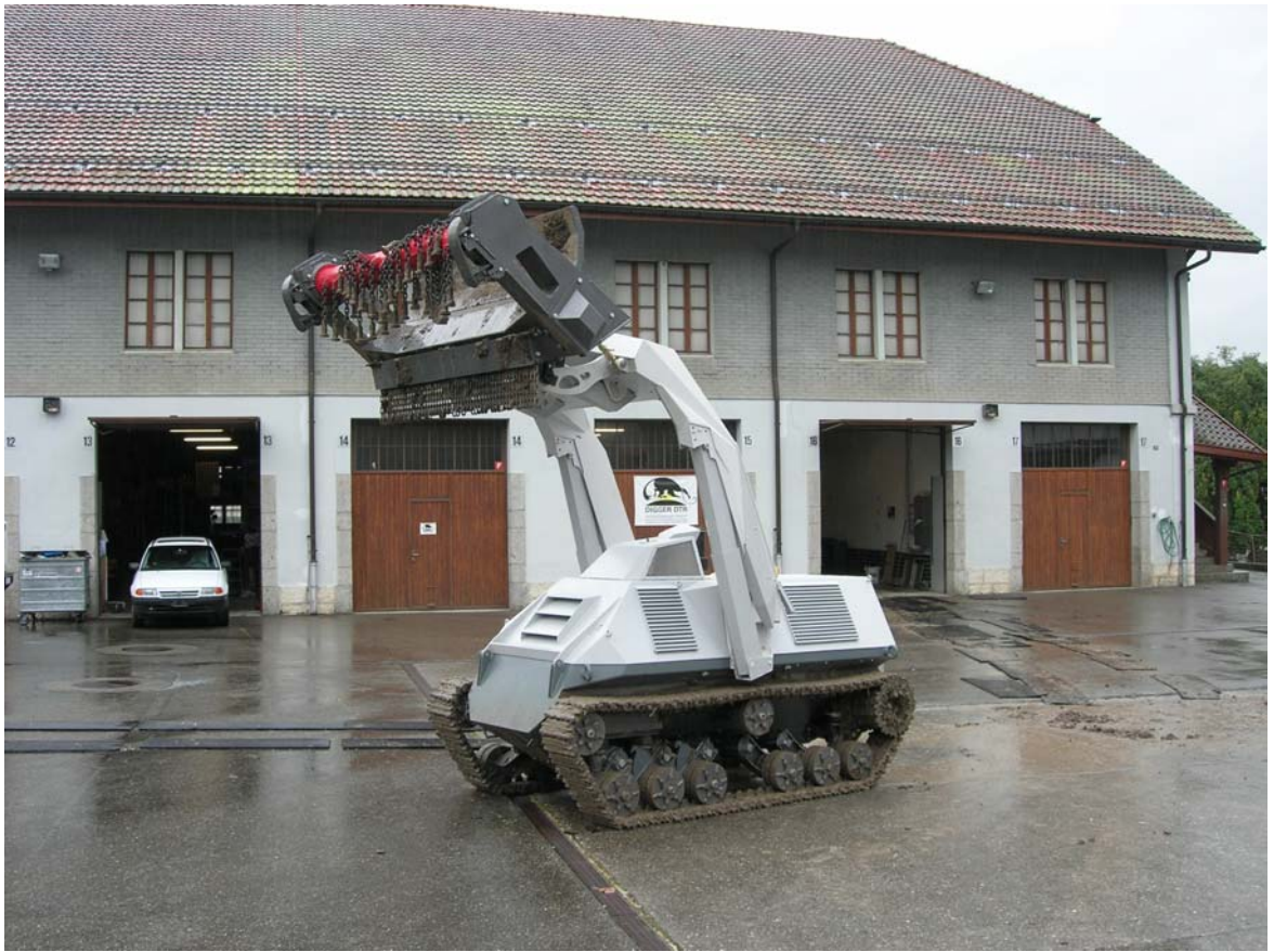
Figure 3-1 Digger D2 with flail raised
