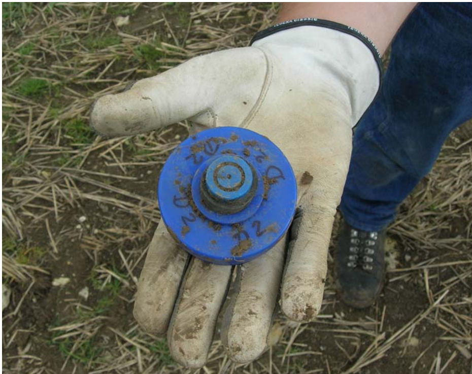
Figure 3-8 WORM mine surrogate as used in runs 4 and 5.
