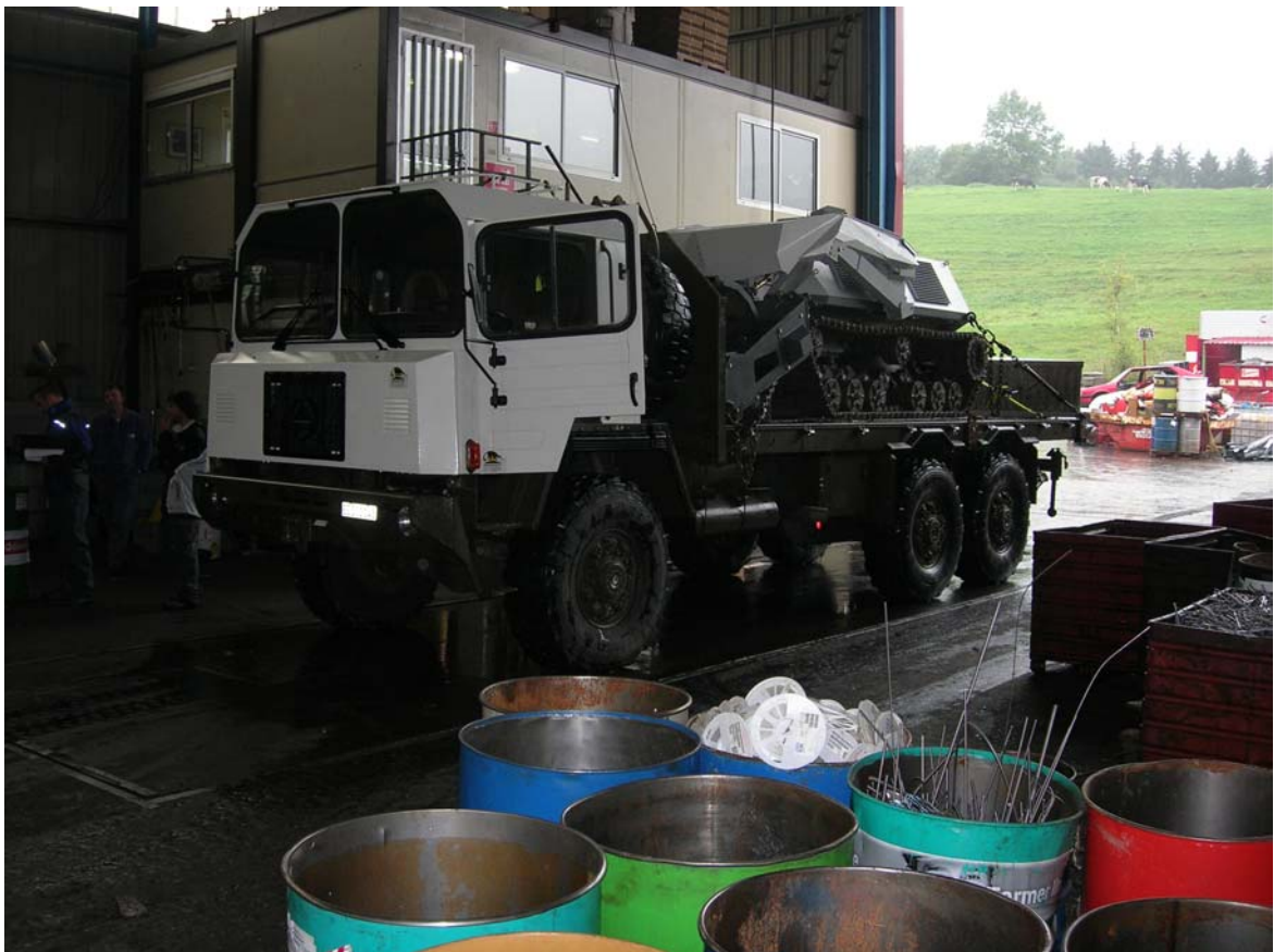
Figure 3-2 Digger D2 and truck -on the weighbridge
