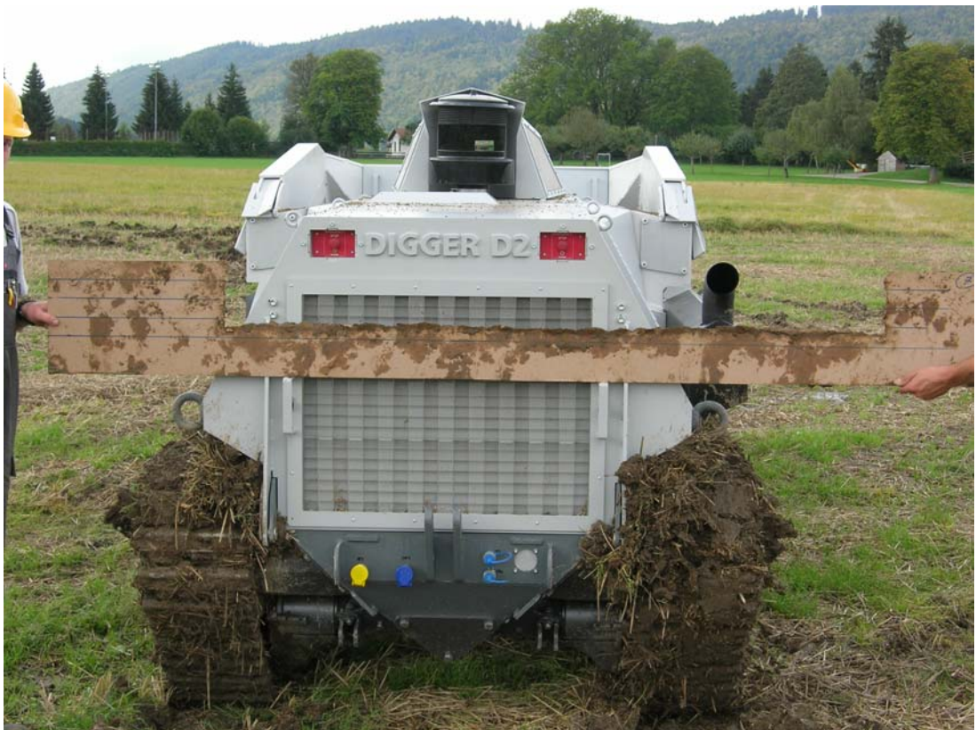
Figure 3-13 Board no. 7 (from run 3) showing a clean-cut profile at just over 15cm
