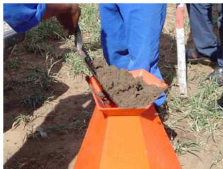
Figure 5.5. Pouring cement mix into mould
