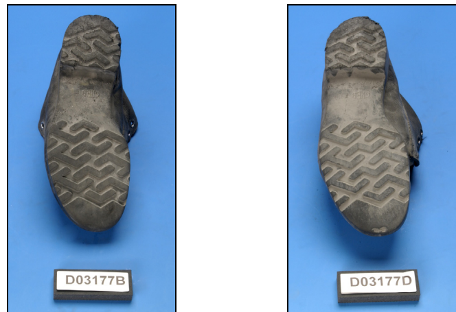
Figure 5. Boot damage with standoff of 175 mm (left) and 125 mm (right)
