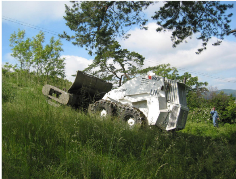
Figure 5-4: B4 MMCS climbing up the grass slope
