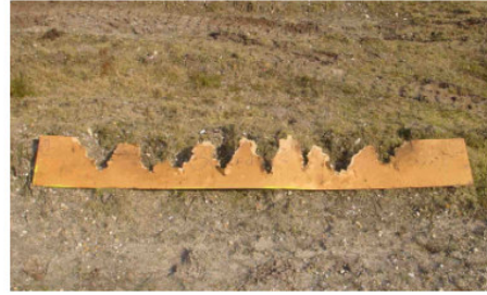
Figure 5-8: Example of an inconsistent cut across the width of the flail
