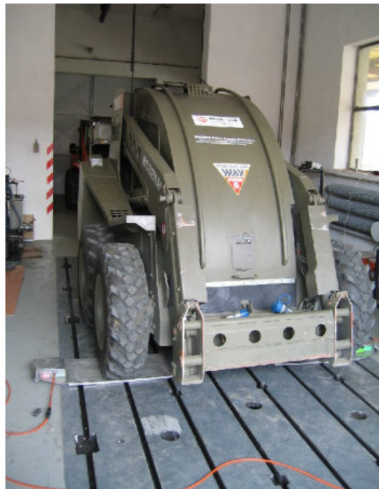
Figure 5-2: B4 MMCS on the load cells (without flail unit)
