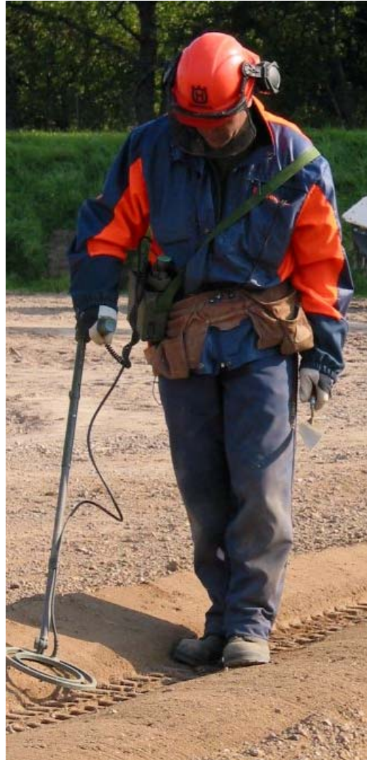
Figure 10. Locating Untriggered Fuzes After The Machine
