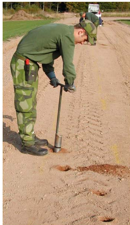
Figure 9. Mine Target Burial Tool To Minimize Soil Disturbance.
