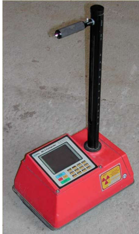
Figure 3. MC-3 Portaprobe for Measuring Soil Compaction and Moisture Content
